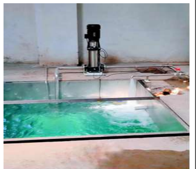
Fig 4: Immersion tank for IP X7 & X8
