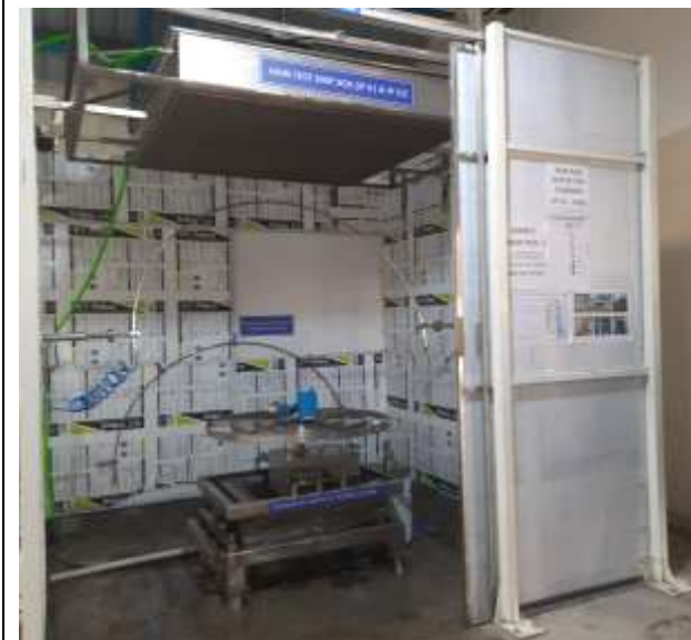
Fig 3: Water testing facility (IP X1- IP X6)
