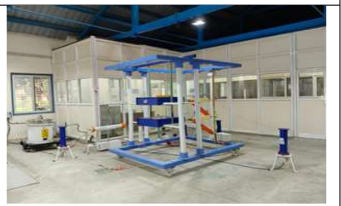
Fig 6: Dielectric test facilities for IP acceptance
