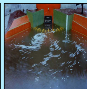
Flow near Power Intake
